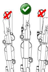
Adjust the long tube with the rear of the butt and tighten a bit more the screw.
