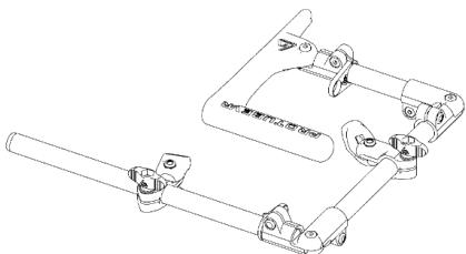
Bend all the connections at an angle of 90° so that the MagTube Rifle almost forms a square.
