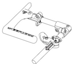
By untightening the butterfly screw, slide the magnetic bracket attachment out.
