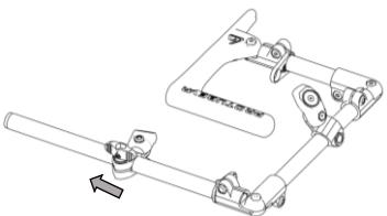
By untightening the lower butterfly screw, slide the magnetic bracket attachment out.
