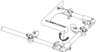
Unscrew the connection on the medium tube closest to the longer tube.
